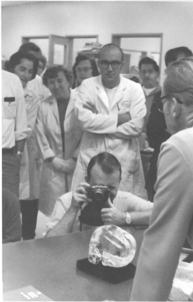
Jim Pruett, components manager on Santa Clara's Frequency Standards team, reviews one of the polarized-light setups used to test the skull. Later, the quartz crystal object was immersed in an index-matching fluid that allowed polarized light to reveal veils and crystalline structure.
