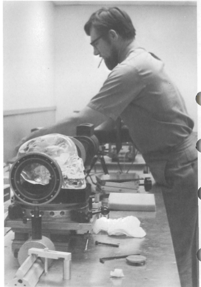
Jim Pruett, components manager on Santa Clara's Frequency Standards team, reviews one of the polarized-light setups used to test the skull. Later, the quartz crystal object was immersed in an index-matching fluid that allowed polarized light to reveal veils and crystalline structure.
